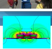
flaws in the superconductor allow enough magnetic flux lines through to make a magnet hover and levitate in place a short distance above the superconductor.
