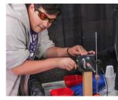
Students explored this property by placing metal rings on an electromagnetic coil and launching the ring like a small cannon!
